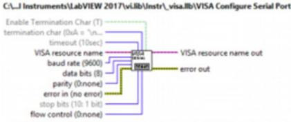
Figura 13. El Configure Serial Port.
